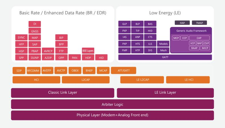
BlueWiz Baseband is a hardware firmware solution that consists of Firmware (HCI+LM+LC+LL (BR/EDR + Bluetooth LE)) and Hardware Accelerator (BR/EDR + Bluetooth LE).
