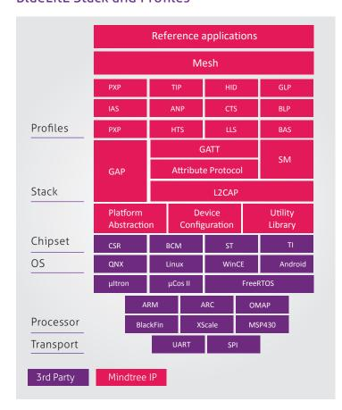
BlueLitE-SP (Stack and Profiles) is designed to be easily portable across a variety of processors, chipsets, transport and OS.
