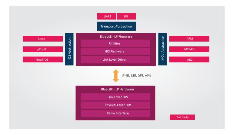
BlueLitE Link Layer is a hardware-firmware co-design. Time-critical functions are handled in the hardware and protocol logics are implemented in firmware. Physical Layer (PHY) is implemented in hardware, performs the GFSK modulation, demodulation, AGC and RSSI measurements.
