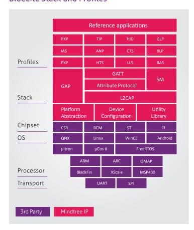
BlueLitE-SP (Stack and Profiles) is designed to be easily portable across a variety of processors, chipsets, transport and OS.
